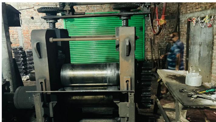
Figure 8. Rolling mill
